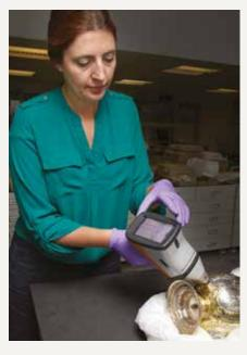
© Conservator demonstrating use of the X-ray fluorescence spectrometer.
